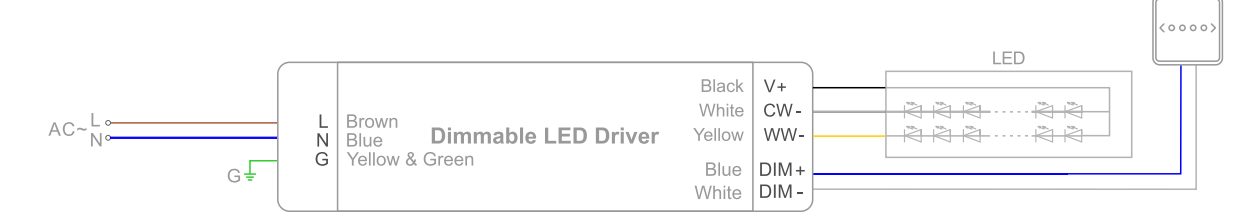
Diagram 6 0-10V/ 1-10V/ 10V PWM/ Potentiometer Dimming ( CCT 2CH ) (The driver is independently connected to the input.)
